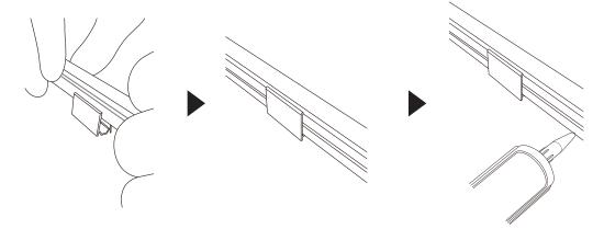
Note 1 : LEDs on FPB , Flexi LED and F Matrix board are vulnerable to pressure while attaching. Please make sure to handle product gently and not to put direct pressure on LEDs and other electronic components.
