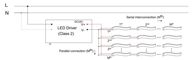
. LED Driver + Flexi LED (with controller , dual white)
