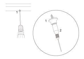
Assemble metal cable grap (2) on the screw mount(1)
