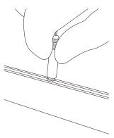
Level the fixture by cutting and adjusting the metal cable.
