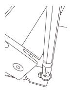
Note 1: Use suitable screw type depending on the surface material. Recommeded base material is metal plate or wood. Materials such as stone, bricks, concrete or drywall need special attention on selection of screw and prior preparation.
