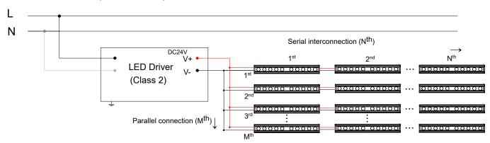
. LED Driver + QPB series (with controller, dual white)
